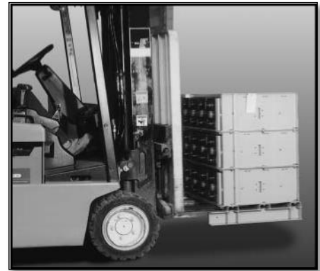
Figure 6-1 Installation Using Forklift
